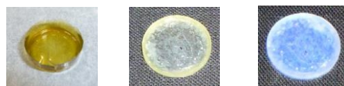
Fig. 1 Photographs of self-standing films of DTG2-PSQ and DTS2-MeS-1 film under room light and UV irradiation at 365 nm (from left to right).
