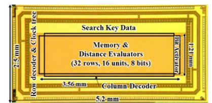
Fig. 2 Search circuit overview of DC and DE for 1 reference vector.
